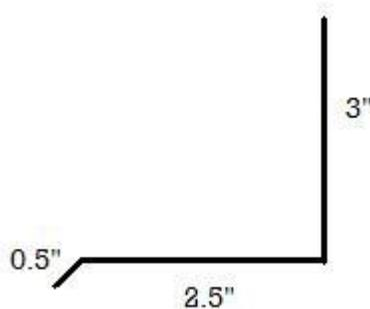
Like the ridge cap, the **ENDWALL FLASHING** can be sealed using outside closures. End-wall flashing is applied where the upward slope of a roof meets a wall. The wall side of the flashing can be covered with siding or counter-flashing, and outside closures are used to seal between the flashing and the panel. Roof slope should be specified when a roof slope exceeds 5/12 pitch.
