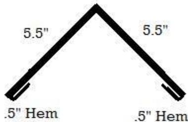
is used to seal the point at which two upward slopes meet. This can be both along the ridge of the roof as well as a covering for a hip. Either wood-grip or self-drilling lap TEK screws are applied through the ribs of the metal roofing panels. Debris, insects, prevailing rain can find easy access under the ridge cap, so closures are often used to either totally or partially seal the opening. Closures under ridge caps are available in 3 types: solid, vented, and hip valley type.
