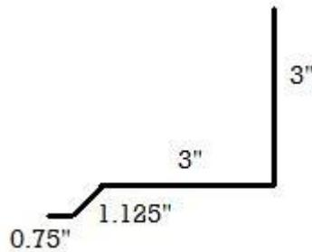
**Sidewall** flashing is applied when the side of the roof butts up against an adjacent wall. The wall-side of the flashing can either be covered over with siding or sealed with counter-flashing. Butyl tape should be applied where the "foot" of the flashing attaches to the roof, and, if used, along the top edge of the counter-flashing.
