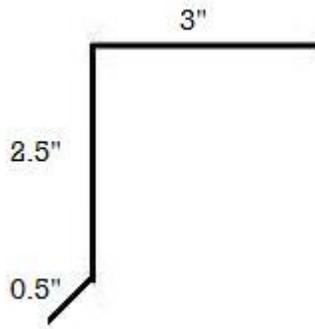
For custom eave drip, specify the amount of the eave that will be covered, and, for steeper roofs, specify pitch. If fascia is desired, specify the dimension you order will be concealed by the eave drip.
