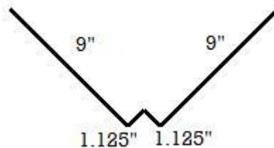
Preformed valleys use a diverter to prevent water from rushing under panels on the opposite side therefore channeling water off the roof. Expanding foam closures are generally used to assure a good seal.
