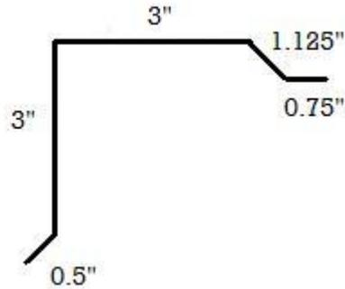
Gable flashing is used to trim the edge of the roofing panel at the gable end of the roof. It should match the eave drip extends along the drip edge of the roof. If the panel is allowed to hang over the gable end, eave drip can be used as an alternative. Butyl tape between the trim and panel eliminates potential leaks.
